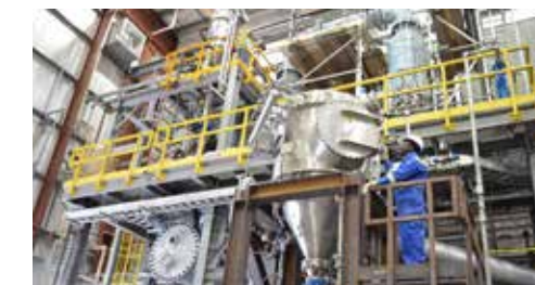
17 Advanced Energy Research Facility Tests diverse waste feedstocks for gasification and production of ethanol and methanol.
