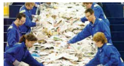
5 Materials Recovery Facility (MRF) Sorts and processes recyclables collected in Edmonton's Blue Bag, Blue Bin and Recycling Depot programs.
