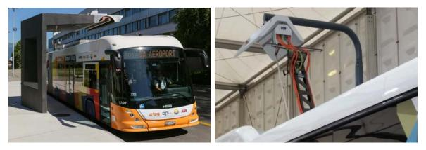
While there are less well-known pantograph systems, with the agreement recently concluded in Europe, they are unlikely to progress past the prototype stage. It should, however, be noted a wide variety of presentations of these two types of pantographs exist; and many of them are aesthetically appealing, enabling City planners to integrate them with other street furniture.
