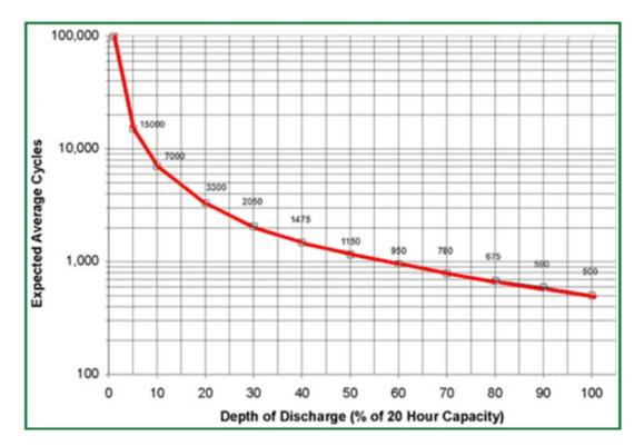
Figure 1 - Sample Cycle Life vs. Depth-of-Discharge Graph
