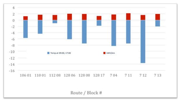
Figure 3.7 Energy Use by Route at Temperature Bus #6011
