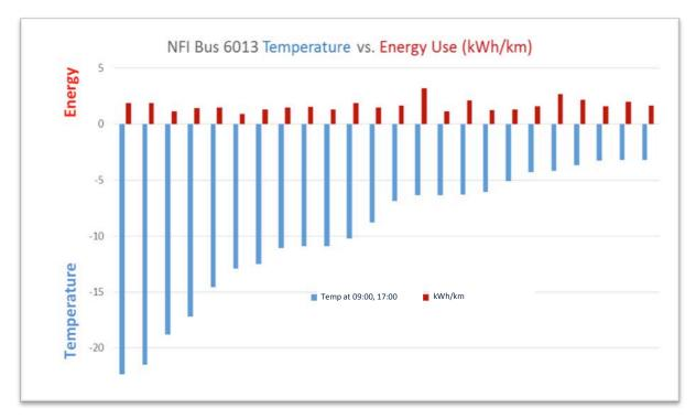
Figure 3.5 Temperature vs. Energy Use for NFI E-bus
