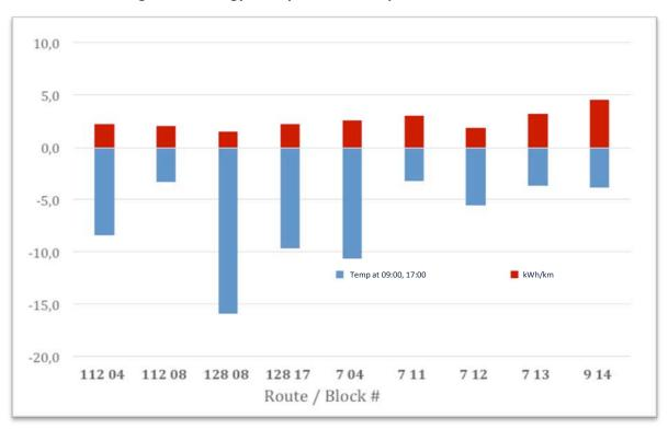
Figure 3.8 Energy Use by Route at Temperature Bus #6013
