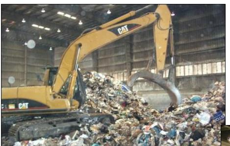
A large backhoe with a grapple loads the waste onto conveyor belts for the trip to the sort room.
