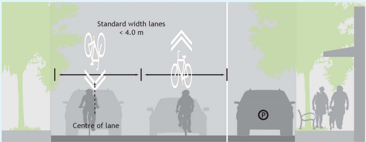
Shared Use Lane Markings for In-Line travel on Regular Lanes
