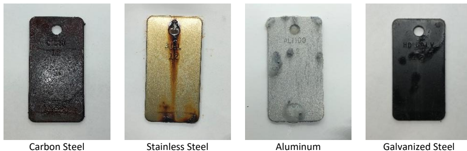
Figure 34 - Modified NACE TM0169 Coupons from Solution 2 (As-Received CaCl 2 Brine)
