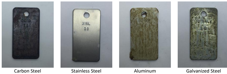
Figure 30 - Standard NACE TM0169 Coupons from Solution 10 (Inhibited \text{CaCl}_2 Brine Diluted 3:97 with Distilled Water)
