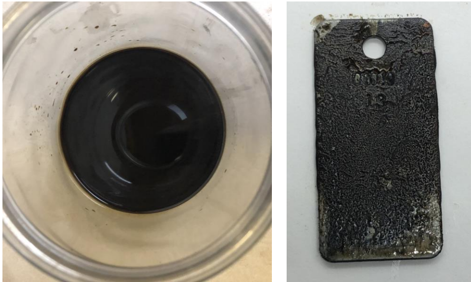
Figure 46 - Effect of As-Received Inhibited \text{CaCl}_2 Brine (Solution 3) on Carbon Steel
