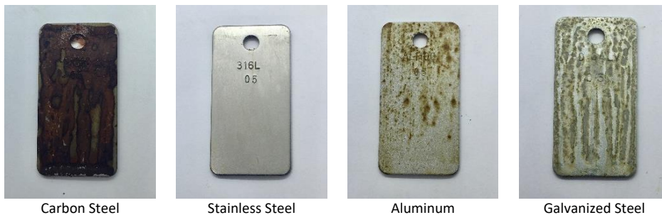
Figure 25 - Standard NACE TM0169 Coupons from Solution 5 (Solution 4 Diluted 1:1 with Distilled Water)
