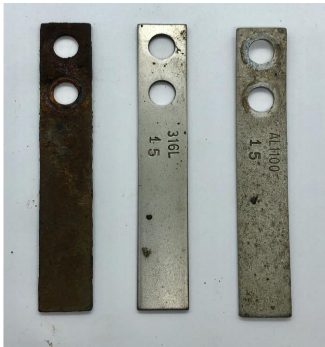
Figure 16 - Lightly Cleaned Field Coupons Recovered from City of Edmonton Buses (Anti-Icing Pilot Program)
