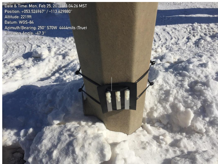
Figure 7 - Coupon Installed on a Lamp post
