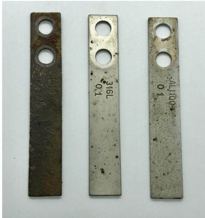
Figure 15 - Lightly Cleaned Field Coupons Recovered from Spruce Grove Buses (Existing Program)
