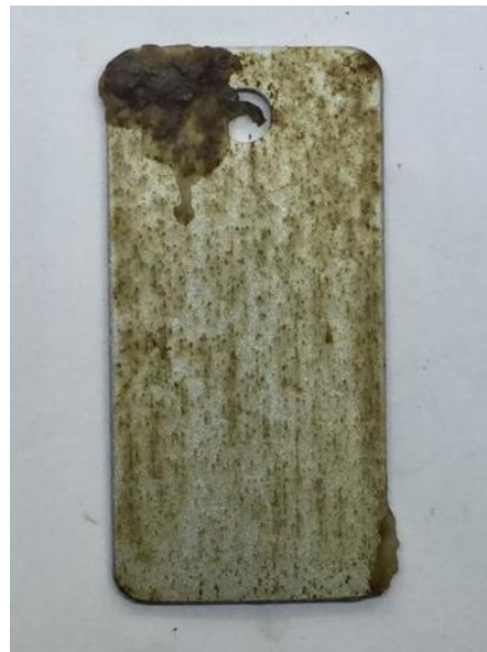
Figure 32 - Biological Buildup on Coupons in Inhibited \text{CaCl}_2 Brine Solutions
