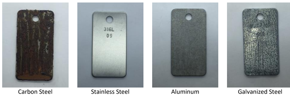
Figure 29 - Standard NACE TM0169 Coupons from Solution 9 (CaCl 2 Brine Diluted 3:97 with Distilled Water)
