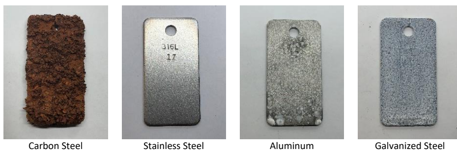
Figure 39 - Modified NACE TM0169 Coupons from Solution 7 (Tap Water)
