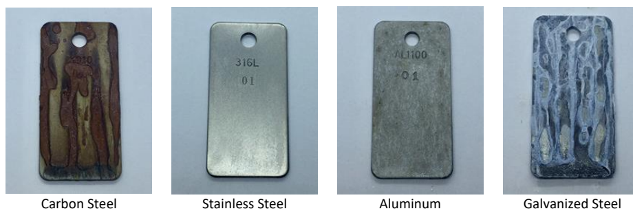
Figure 21 - Standard NACE TM0169 Coupons from Solution 1 (Saturated NaCl)
