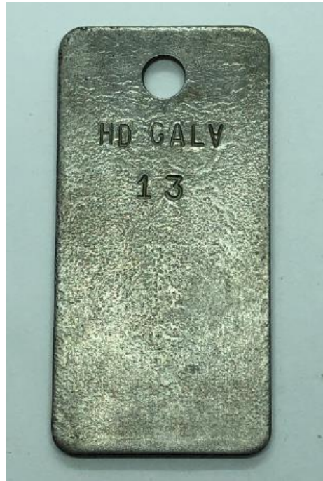
Figure 55 - Zinc Coating Entirely Consumed from Inhibited \text{CaCl}_2 Brine (Solution 3)
