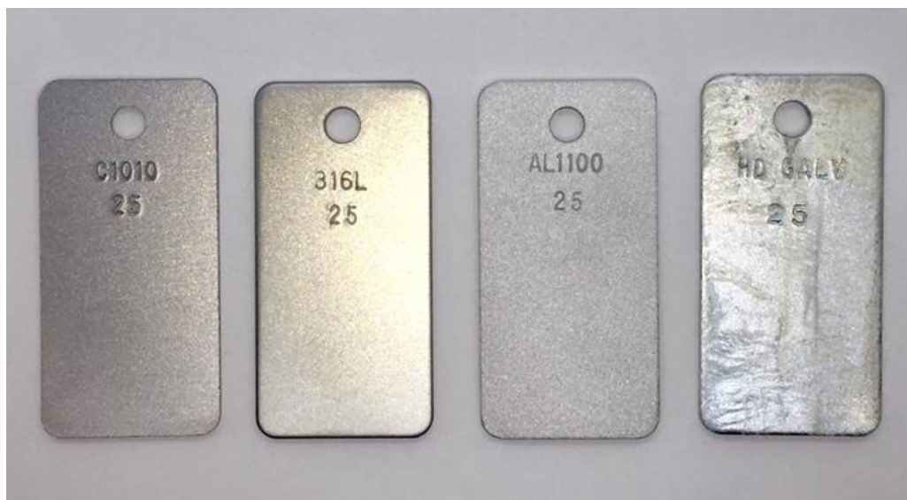
Figure 18 - As-Received Laboratory Coupons
