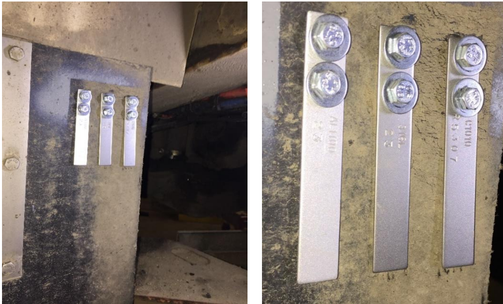
Figure 5 - Coupons Mounted on Bus Mud Flaps
