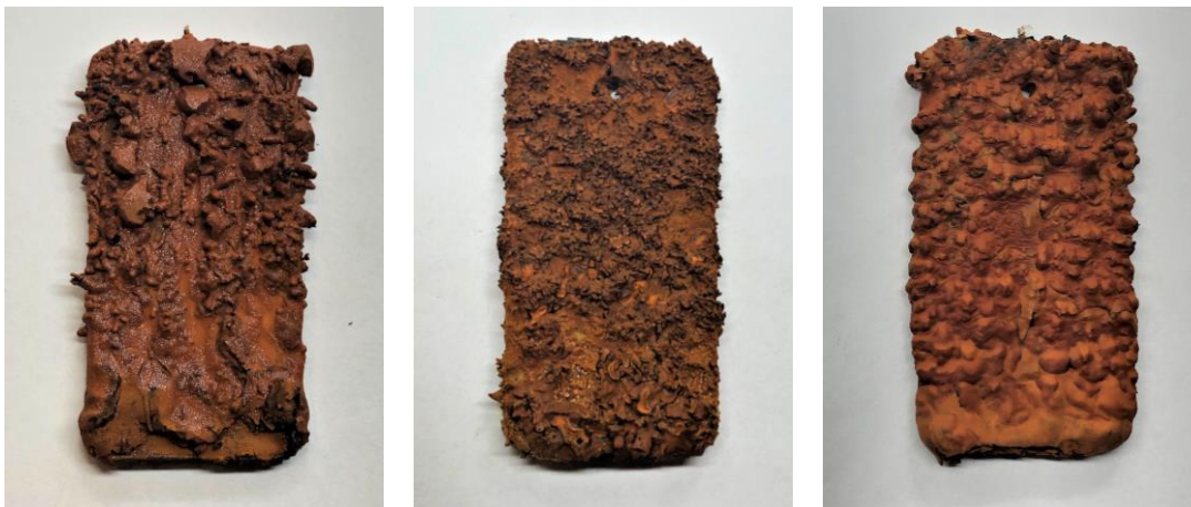
Figure 48 - Corroded Carbon Steel Coupons (From Left to Right: Solution 6, 7, and 9)
