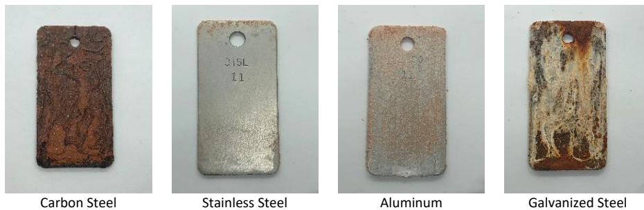
Figure 33 - Modified NACE TM0169 Coupons from Solution 1 (Saturated NaCl)
