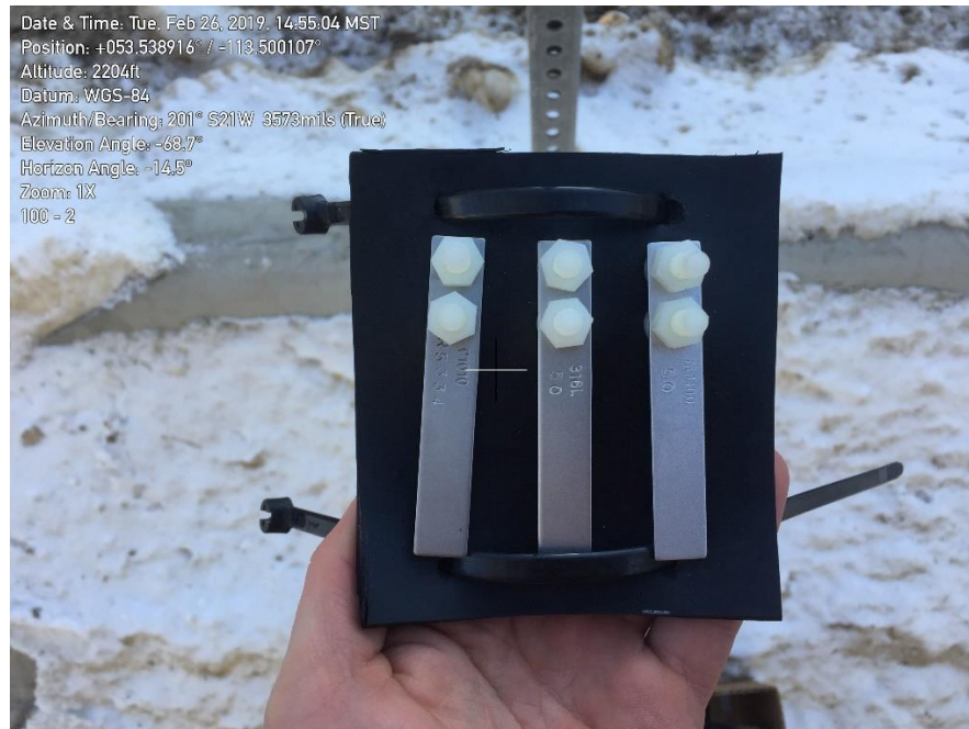
Figure 6 - Field Coupon Mounting Apparatus
