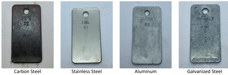
Figure 22 - Standard NACE TM0169 Coupons from Solution 2 (As-Received \text{CaCl}_2 Brine)
