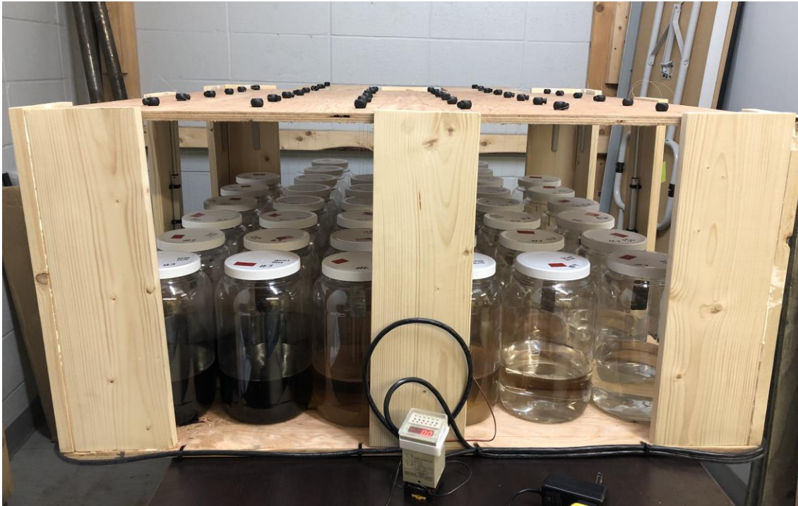
Figure 19 – Side View of the Laboratory Setup (Coupons Out of Solution)
