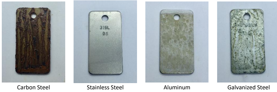
Figure 26 - Standard NACE TM0169 Coupons from Solution 6 (Solution 4 Diluted 3:97 with Distilled Water)
