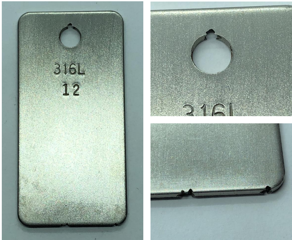
Figure 51 - Stainless Steel Coupon Exposed to \text{CaCl}_2 Brine
