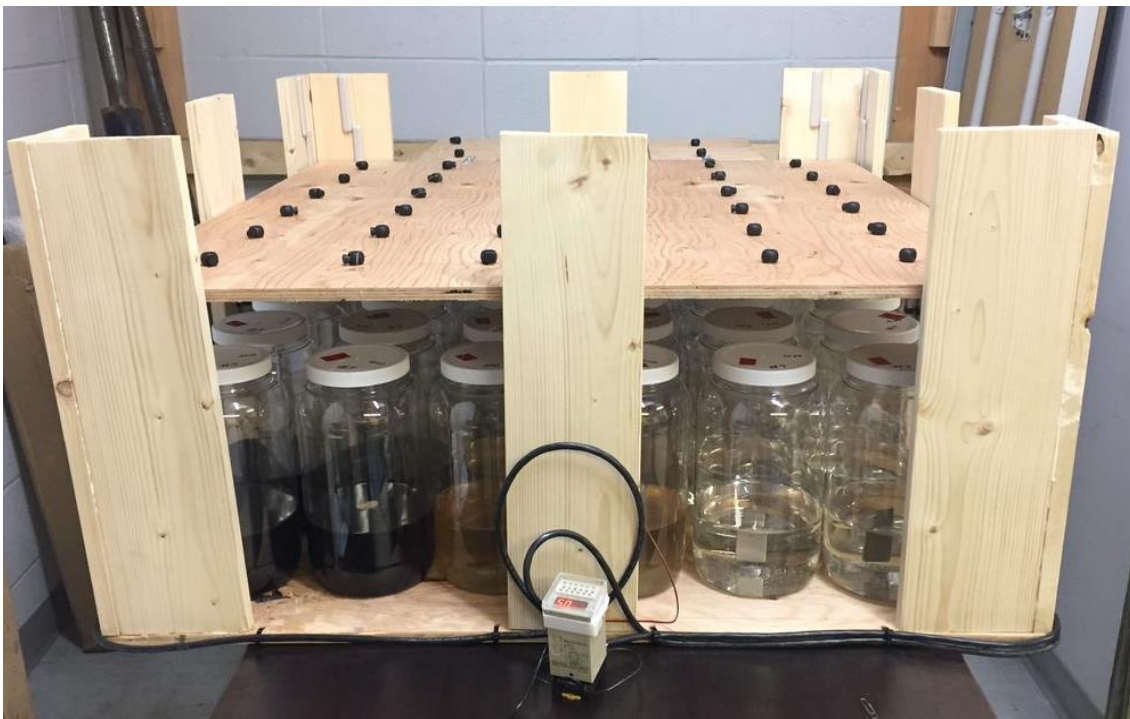
Figure 20 – Side View of the Laboratory Setup (Coupons Immersed in Solution)
