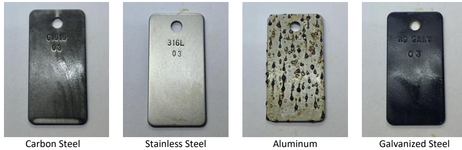
Figure 23 - Standard NACE TM0169 Coupons from Solution 3 (As-Received Inhibited \text{CaCl}_2 Brine)
