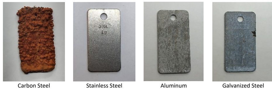
Figure 41 - Modified NACE TM0169 Coupons from Solution 9 (CaCl 2 Brine Diluted 3:97 with Distilled Water)
