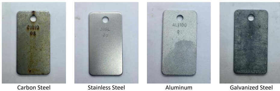
Figure 28 - Standard NACE TM0169 Coupons from Solution 8 (Distilled Water)
