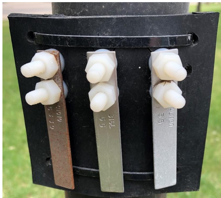
Figure 13 - Control Coupons Outside the Corrpro Office (Environmental Control)
