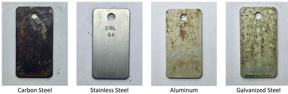
Figure 24 - Standard NACE TM0169 Coupons from Solution 4 (Mixed Solution of Saturated NaCl and Inhibited \text{CaCl}_2 Brine (95:5))
