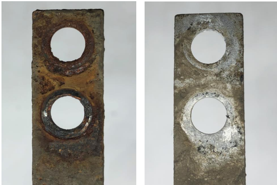
Figure 17 - Crevice Corrosion on Field Coupons Installed on Buses (Carbon Steel on Left, Aluminum on Right)
