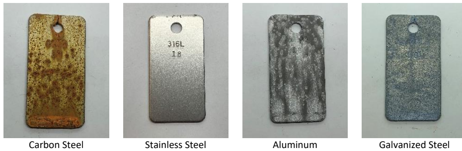
Figure 40 - Modified NACE TM0169 Coupons from Solution 8 (Distilled Water)
