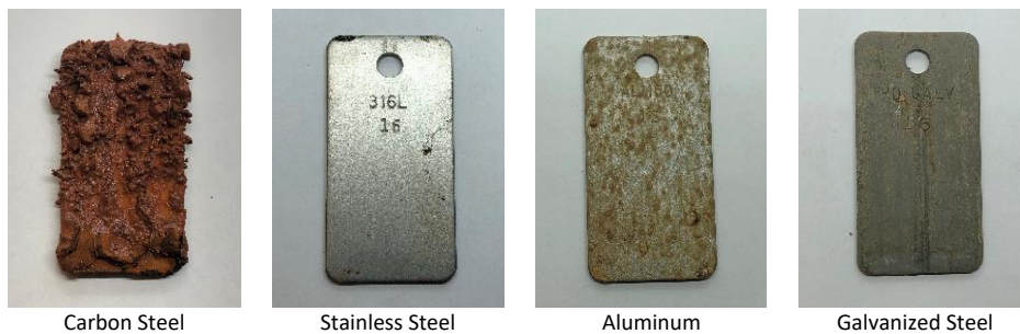
Figure 38 - Modified NACE TM0169 Coupons from Solution 6 (Solution 4 Diluted 3:97 with Distilled Water)
