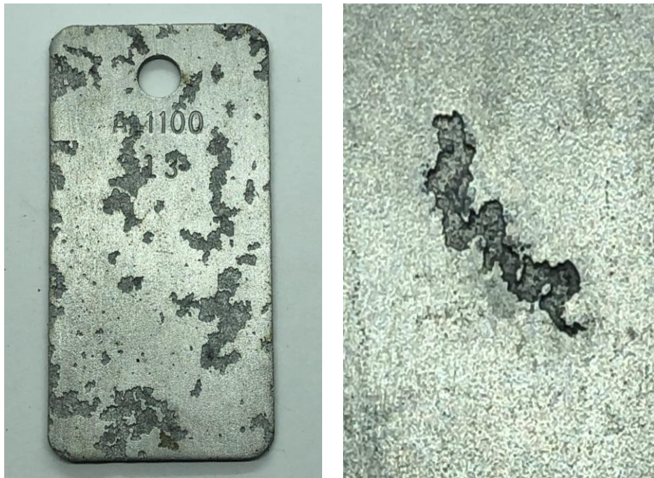
Figure 53 - Pitting Corrosion on Aluminum Coupons
