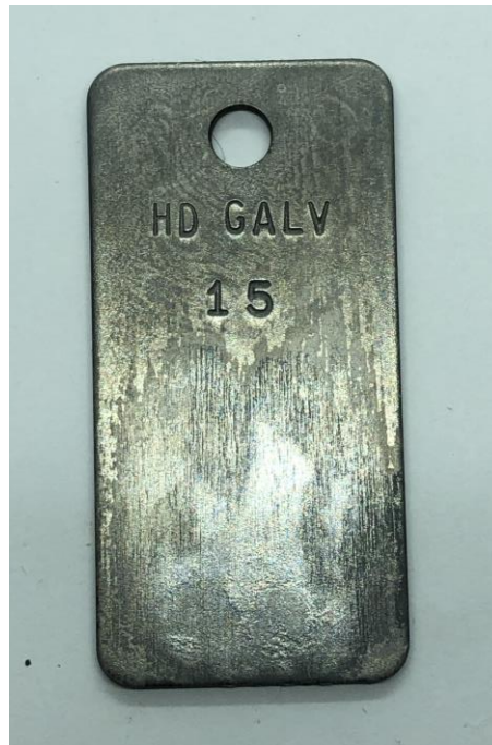
Figure 56 - Zinc Coating Break-down on Galvanized Steel Coupons
