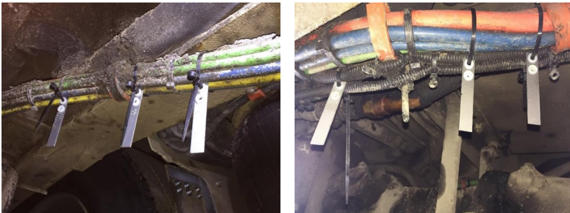
Figure 4 - Coupons Mounted Behind the Wheel Well of Buses
