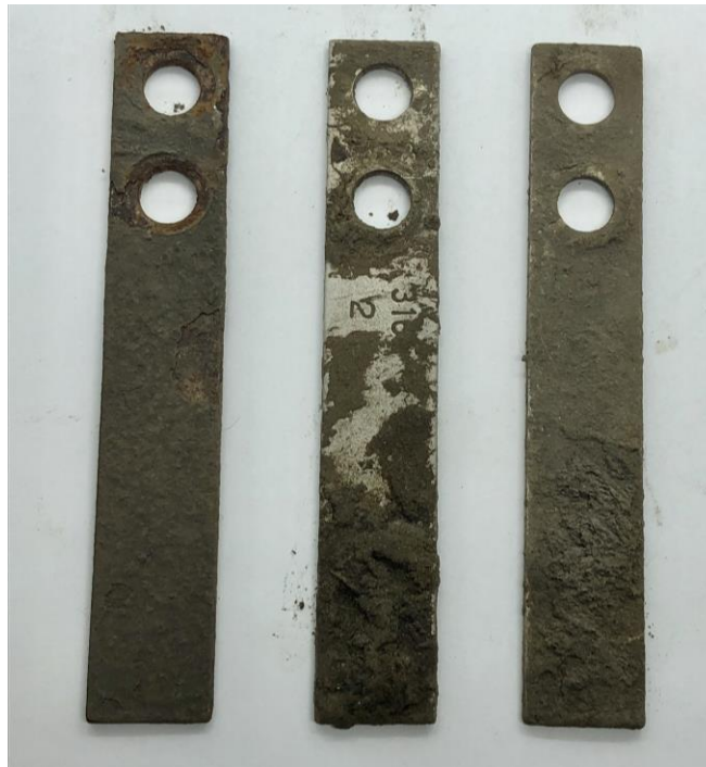
Figure 10 - As-Retrieved Corroded Field Coupons Installed on Buses
