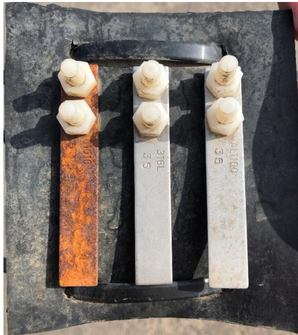
Figure 11 - Infrastructure-Related Field Coupons Retrieved from 122 nd Street (Existing Program)
