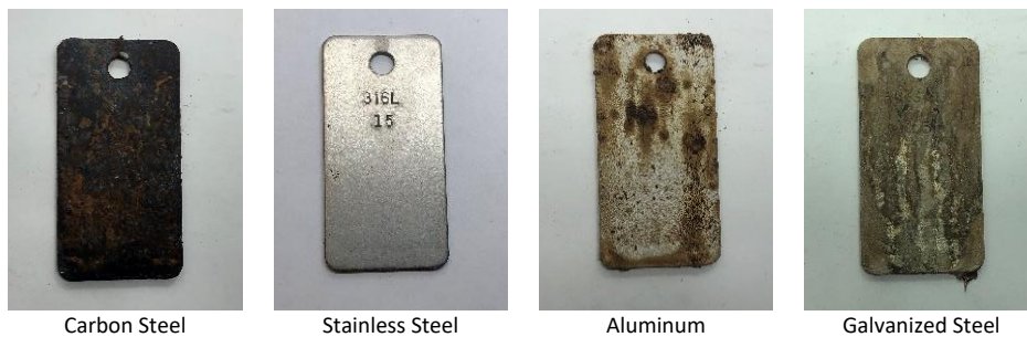
Figure 37 - Modified NACE TM0169 Coupons from Solution 5 (Solution 4 Diluted 1:1 with Distilled Water)
