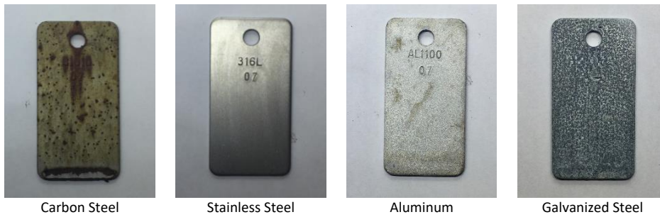
Figure 27 - Standard NACE TM0169 Coupons from Solution 7 (Tap Water)
