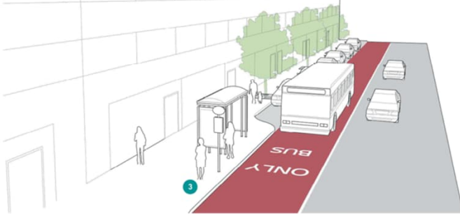
Source: Illustration of a Dedicated Offset Bus Lane
