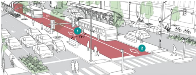
Source: NACTO: Illustration of a Dedicated Centre Bus Lanes
