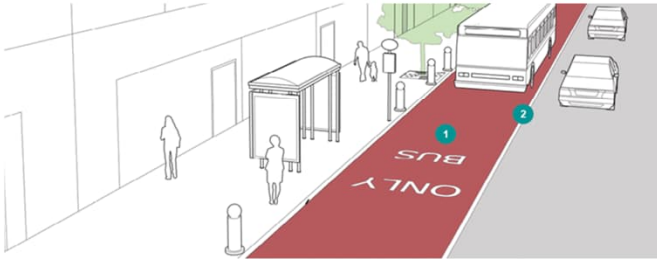
Source: NACTO: Illustration of a Dedicated Curbside Bus Lane
