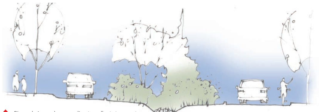
▲ Bioswale in roadway median to collect stormwater.
