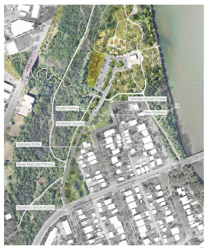
Figure 34. Main Vehicular Access - Plan View
