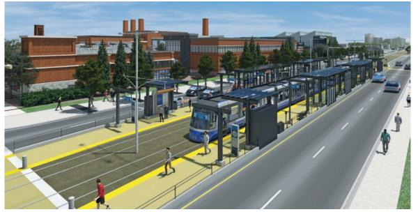
Low-floor LRT vehicles were first introduced in the late 1980s and have since evolved to become the industry standard for new LRT systems in Europe and North America. Most of the mechanical equipment on a low-floor LRT vehicle is located on the roof, which means the train doors open at street level for step-free boarding onto the vehicle.
