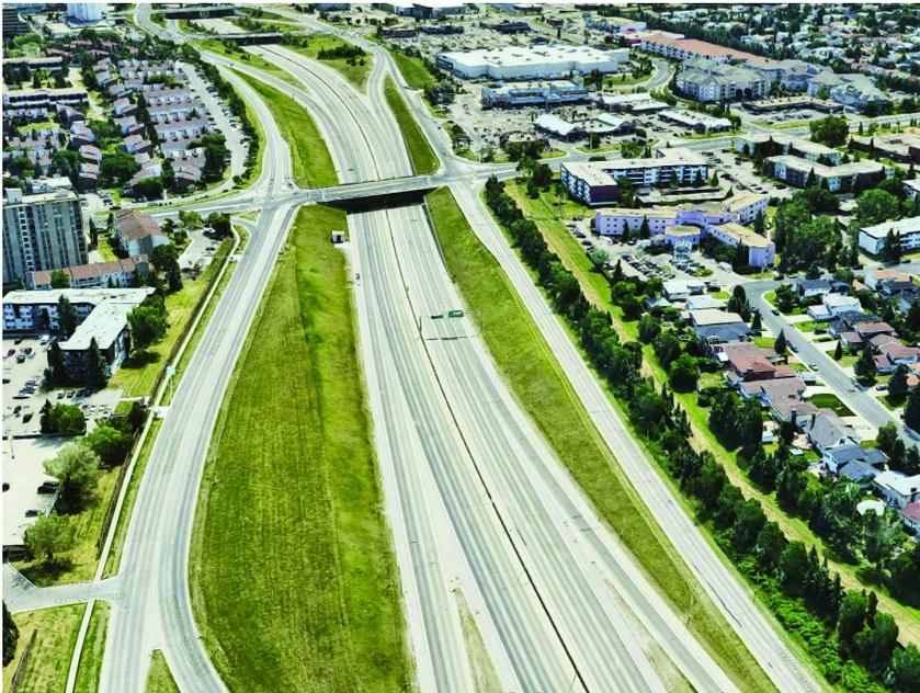
Even using a service road concept, there is insufficient space to develop both on-and off-ramps at all interchange locations.
