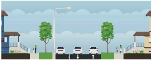
Sidewalk Existing Boulevard On-Street Parking Two-way Traffic Existing Sidewalk Boulevard
