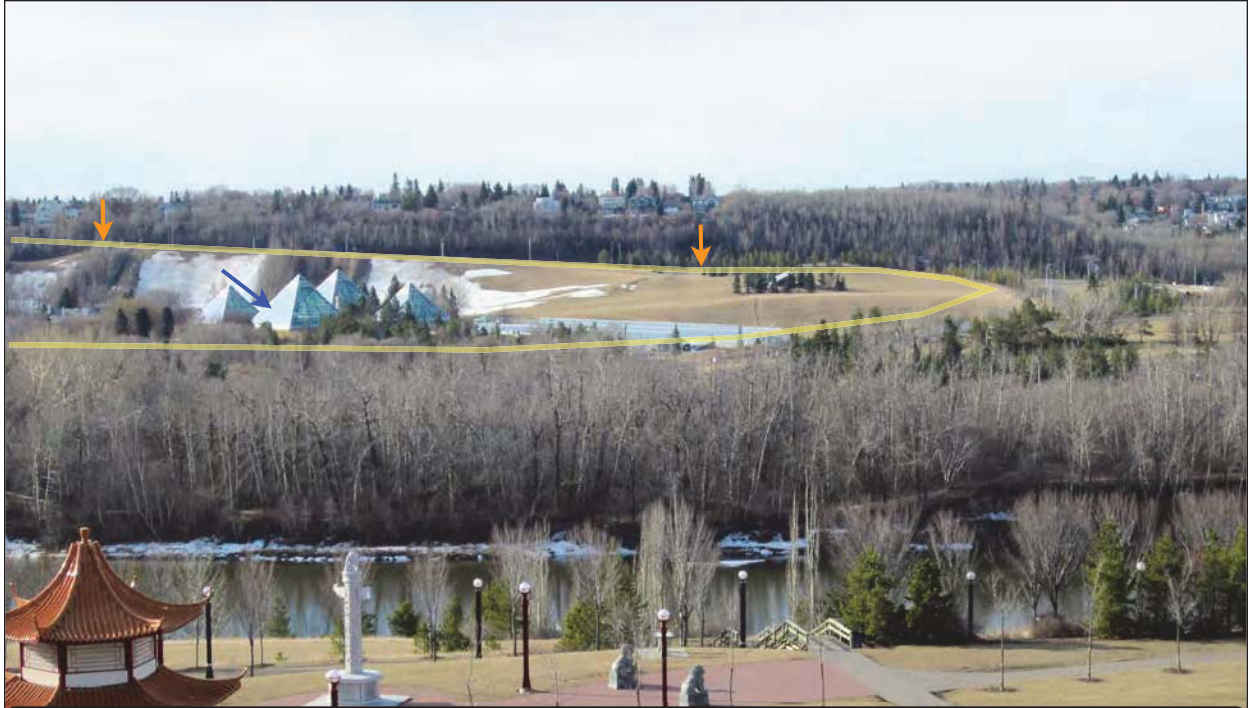
Figure 27. View looking south from top of north valley slope showing Muttart Conservatory pyramids (→), Connors Road (→) and proposed LRT alignment (—). Area between orange arrows (→) is area that bedrock is close to the surface.
