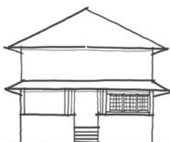
Full-width partially enclosed verandah
