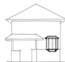
Typical window arrangement - Bay windows on ground level/front facade
