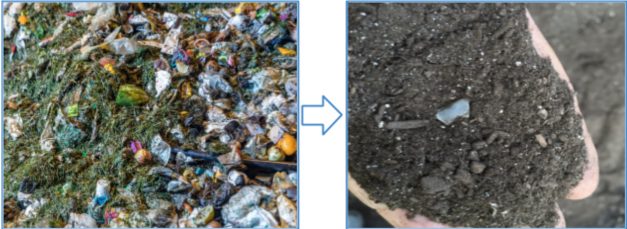
Figure 3: The photo depicts the inbound contaminated waste stream to the ECF, sorted out from the residential garbage stream (left) and the processed compost (right). The lower quality of the end product is visible in the photo on the right.
