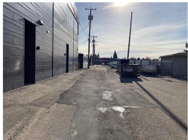
A power line runs along the east side of the alley. Based on on-site observations, the pole locations do not impede traffic movements.
