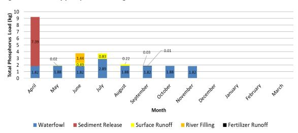
Figure 20. Monthly phosphorus loading to Hawrelak Lake from different sources
