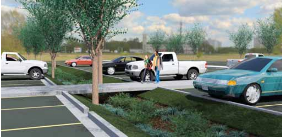
BIOSWALE MEDIAN PERSPECTIVE VIEW
