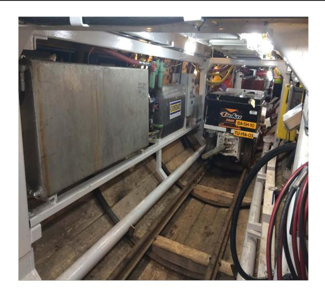
Figure 1c: NEST Stage NC2/NC3- Trailing gear which includes the gantry & conveyor of the TBM
