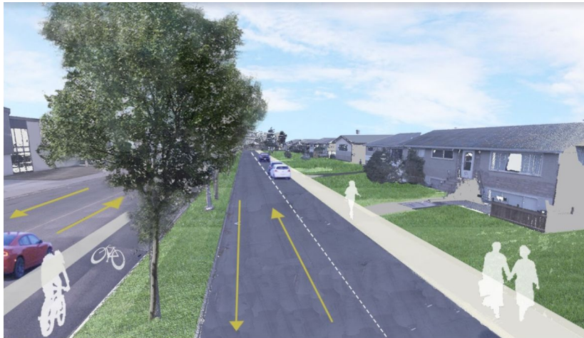
Option for service road to be used for 2 way driving and parking. Sidewalks are less than standard width in most locations or missing. Future bike facilities on 132 Avenue are located beside the driving lane.
