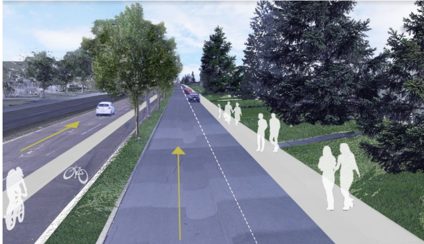
Option for service road to be used for 1 way driving and parking. Sidewalks can be built to standard width and missing sidewalks can be added. Future bike facilities on 132 Avenue are located beside the driving lane.
