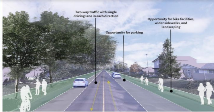
Future one way driving lane in each direction with parking on each side of the road. Opportunity for bike facility, wider sidewalk and landscaping.
