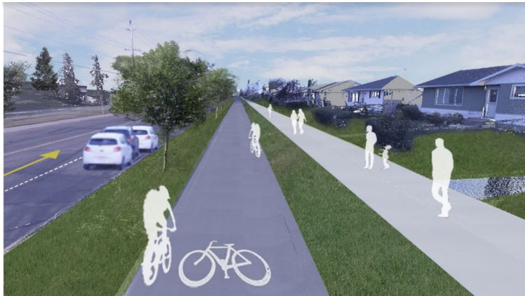
Option for service road to be repurposed to be used for walking, biking and beautification. Sidewalks can be built to standard width and missing sidewalks can be added. Future bike facilities can be located further away from driving lanes. There is room to add landscaping features. Parking is accommodated along 132 Avenue beside the driving lanes.
