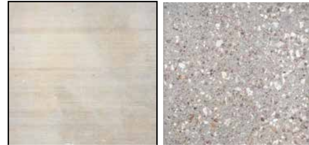
BROOM FINISHED CONCRETE SANDBLASTED BANDS
