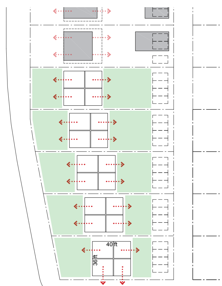
STEP ONE establish 4-pack townhouses sized to fit typical lot | applicable to repeat development maintain domestic structure scale | street facing units with rear units + parking along alley
