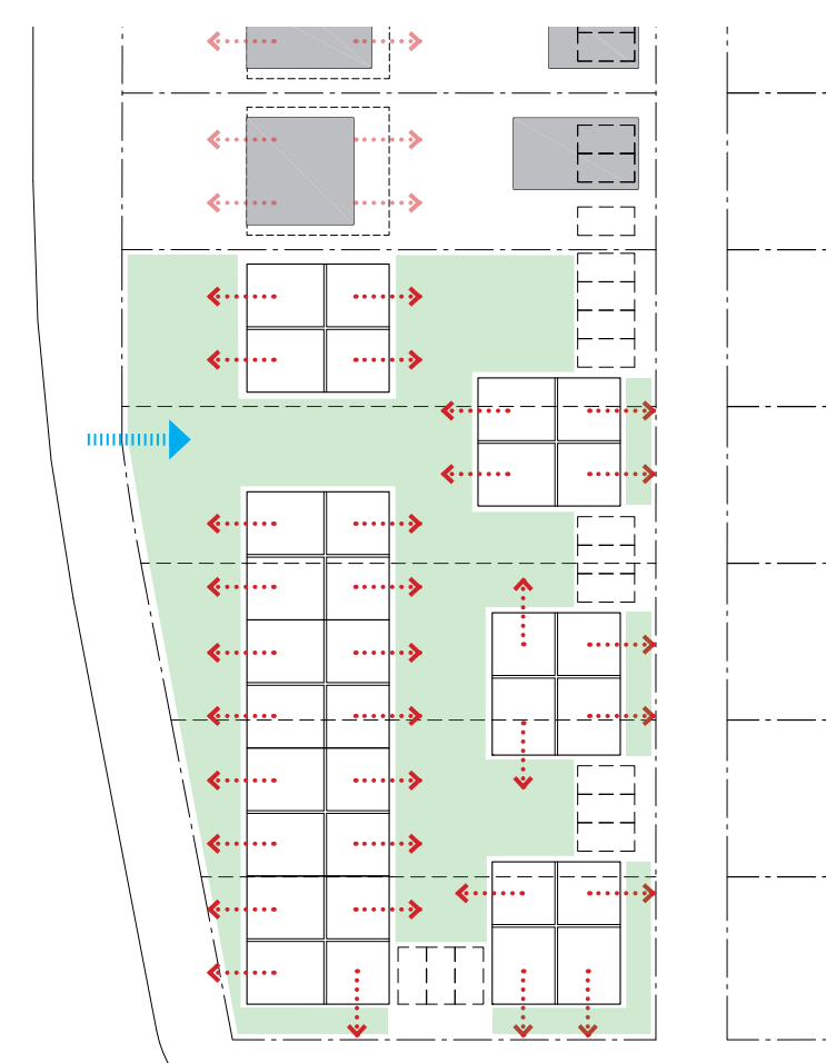
STEP TWO prioritize communal open space between structures | add density with porosity diversify unit types for rental + sale opportunity | redistribute parking into pockets
