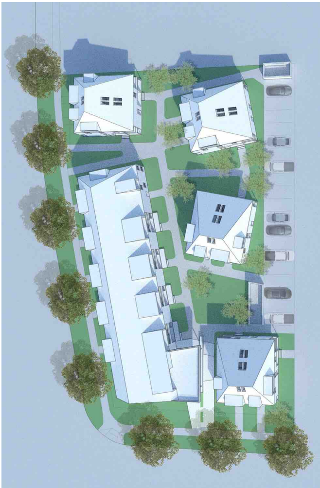
STEP ONE establish 4-pack townhouses sized to fit typical lot | applicable to repeat development maintain domestic structure scale | street facing units with rear units + parking along alley
