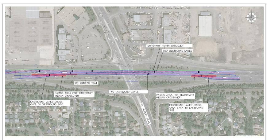
NOTE: TEMPORARY MEDIAN CROSSOVER PLAN PREPARED FOR POSTED 50KM/HR CONSTRUCTION SPEED ZONE ACCORDING TO MUTCD STANDARDS (FIGURE D4042)
