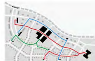
Dispersed Traffic Pattern - Promotes walking and biking - Shorter trip lengths - Dispersion of trips on multiple roadways
