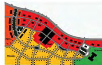
Traditional Development - Roadway network with multiple connections - Proximity of uses - Public spaces link community
