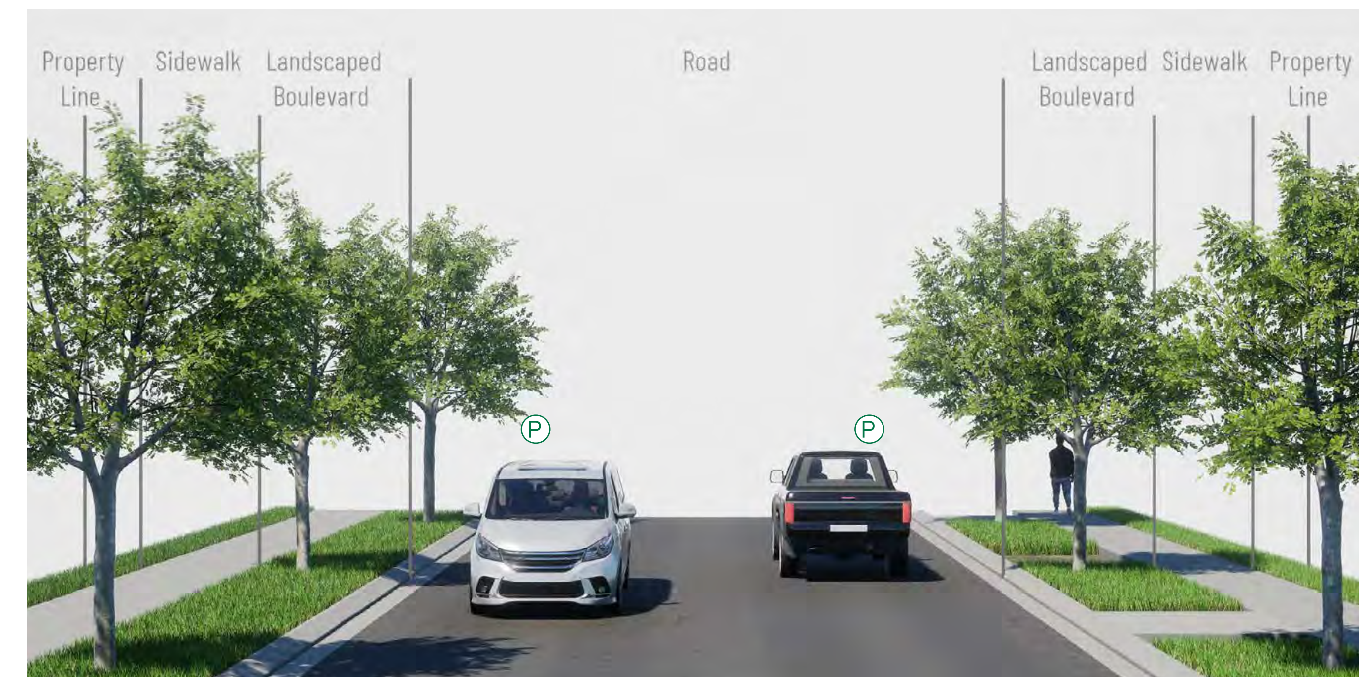
Scenario C: Sidewalks with landscape boulevards on both sides of the road. Parking unchanged.
