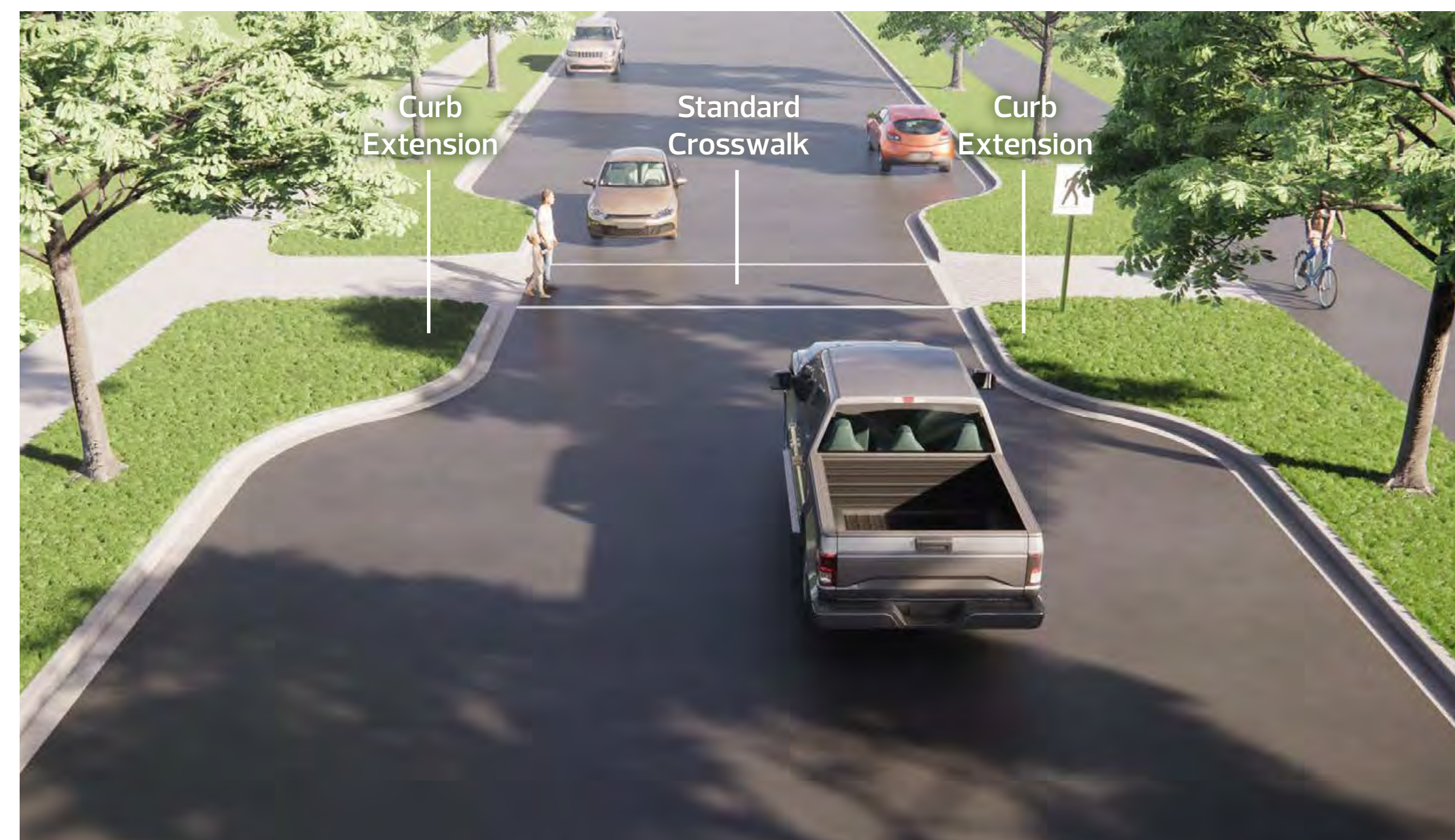
Example of Standard Crossing with Curb Extensions
