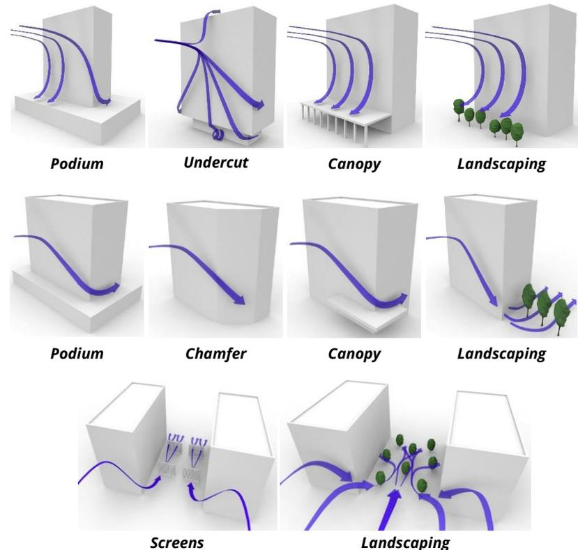
**Image 4b: Examples of Common Wind Control Measures**
