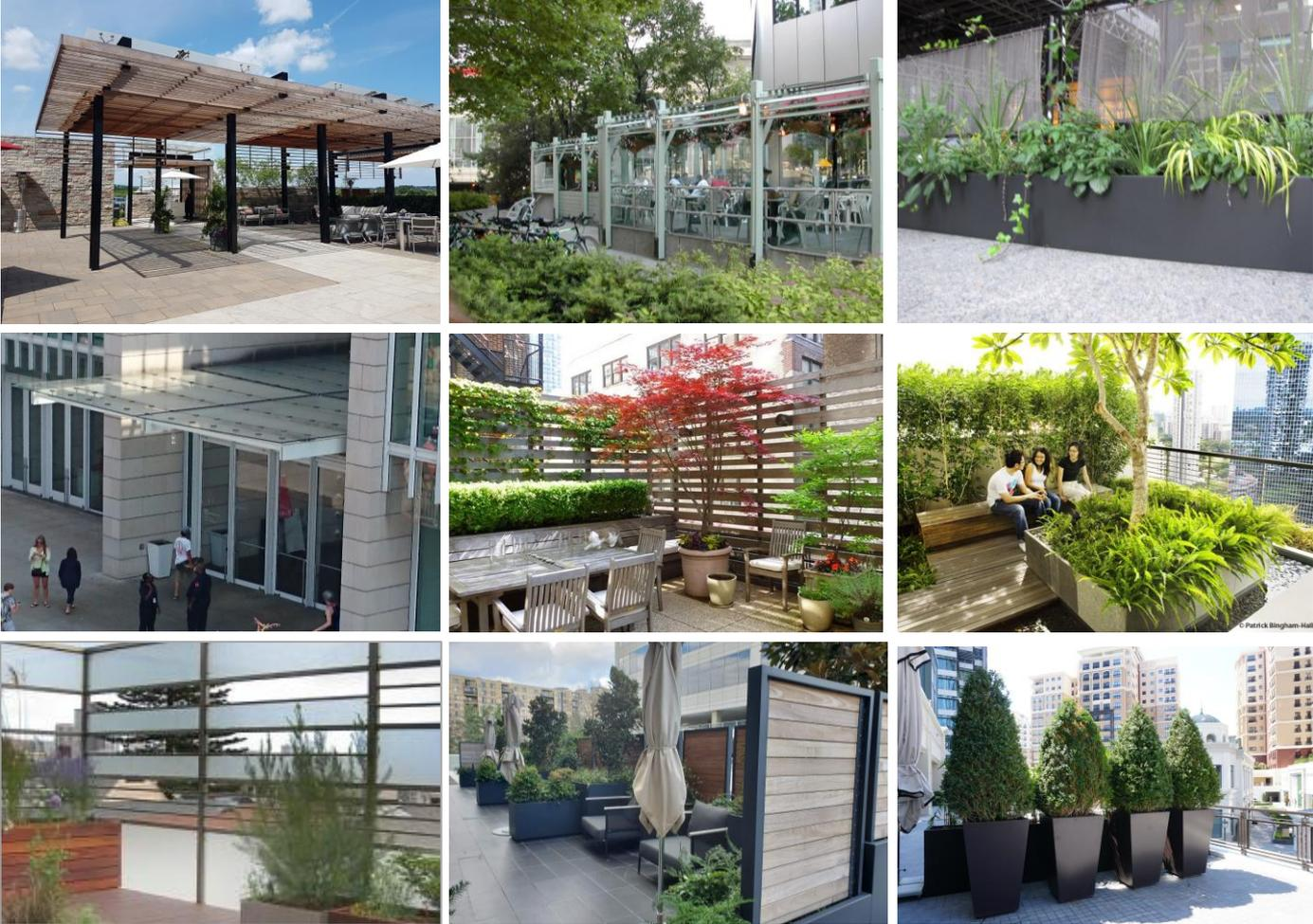
**Image 7: Examples of landscaping, wind screens, trellises and canopies for wind control**
