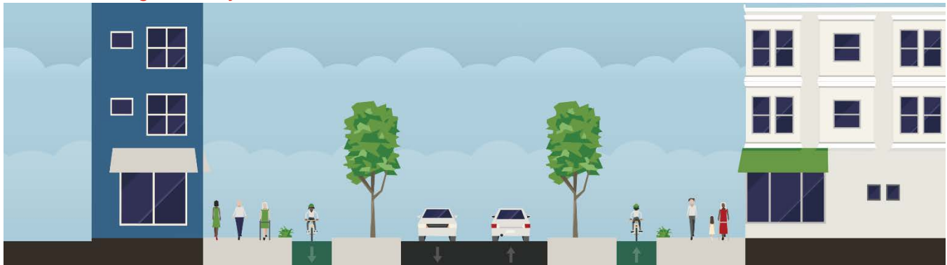
Figure 20: Base 24.4m Right-of-Way Cross-Section
