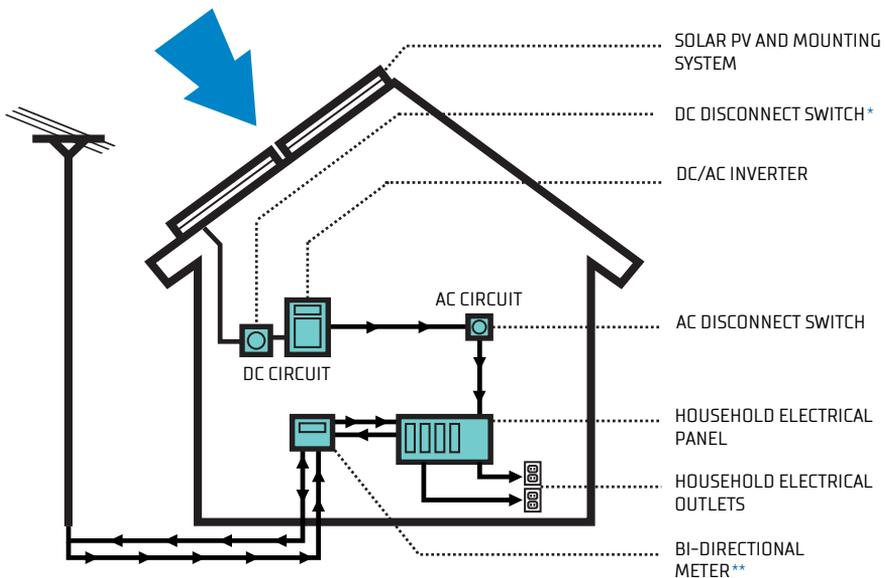
\* The DC Disconnect Switch allows for the inverter to be shut down for maintenance or in the event of a house fire
