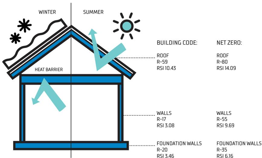
Note that a Heat Recovery Ventilator (HRV)—see **Ventilation Information** chapter—was assumed to be in use for both the building code and net zero R-value examples above; without an HRV, the R-values will typically increase.
