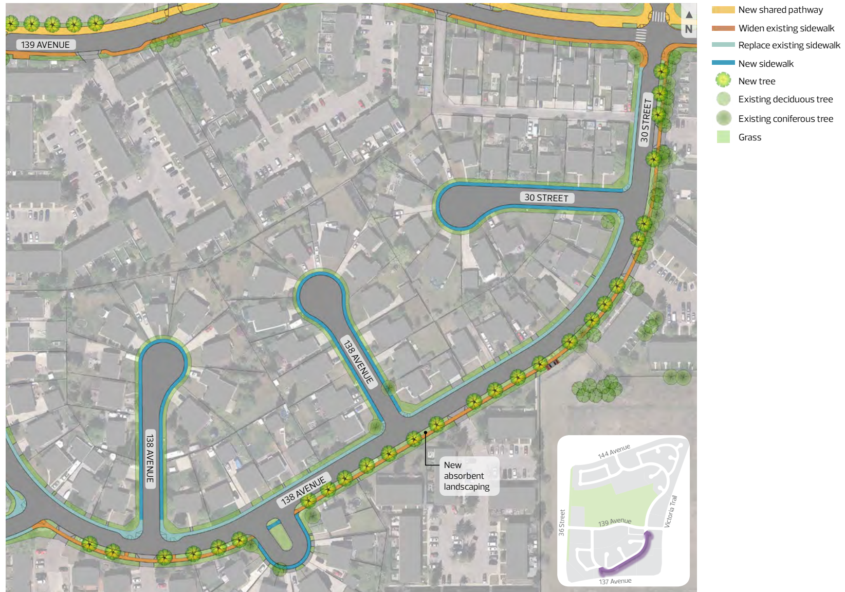
New boulevard along the local loop road of 142 Avenue/30 Street/138 Avenue - Plan: South portion
