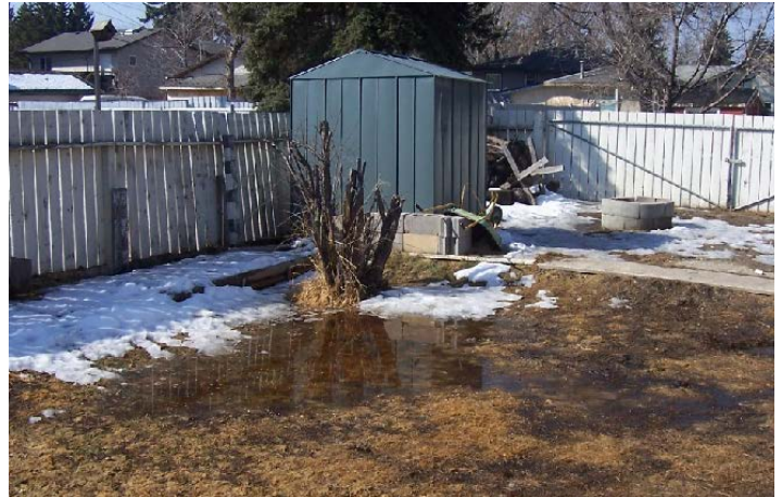
Low areas in the yard can result in pooling and flooding during heavy rain or snow melt
