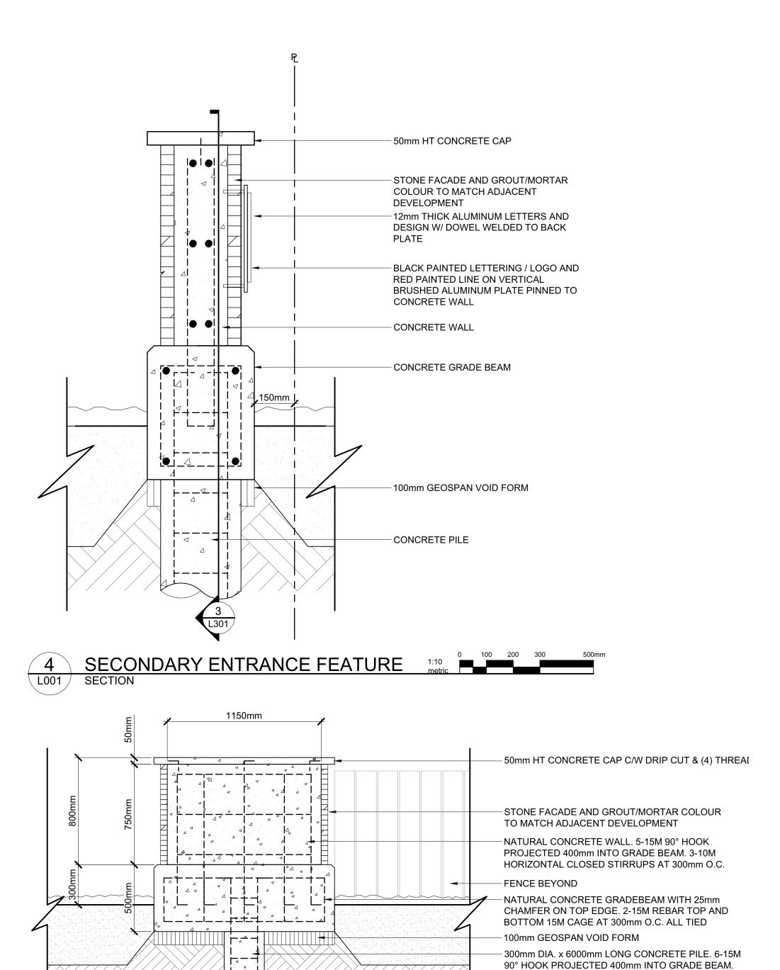
PILE. TOP 600mm OF PILE TO HAVE 150mm O.C. PROJECTING INTO PILE CAP. SONOTUBE TOP 2m OF PILE
