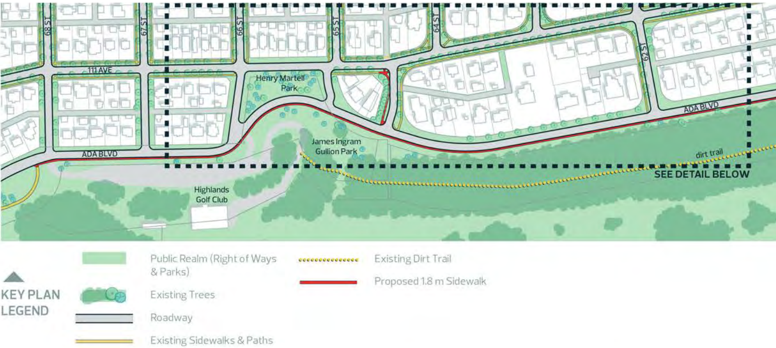
FIGURE 11 – Ada Boulevard Concept 3 – Monolithic Sidewalk
