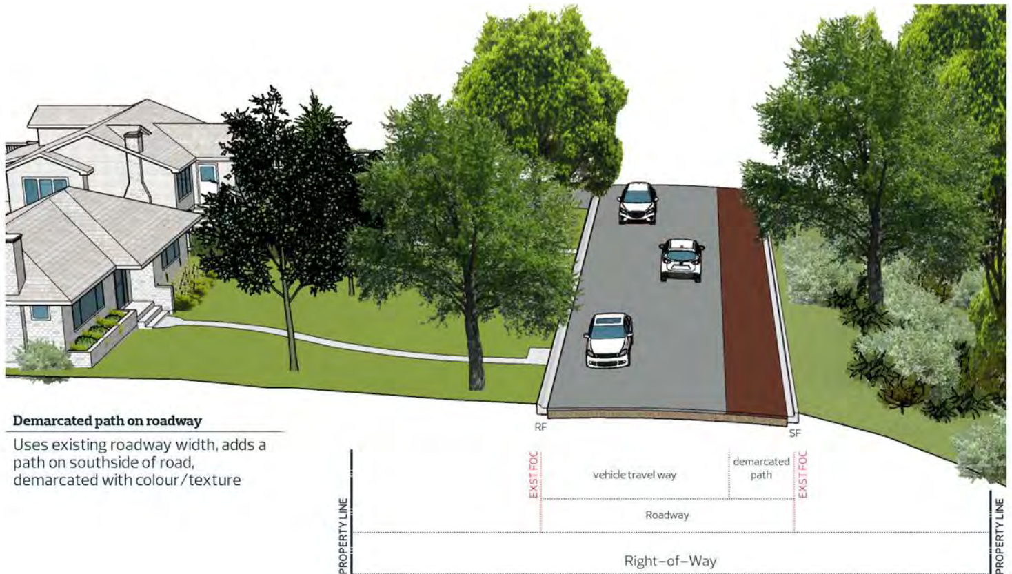
FIGURE 14 – Cross-Section: Demarcated Path
