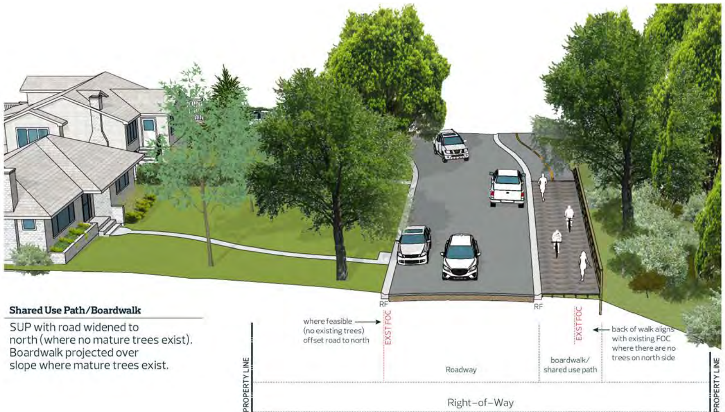
FIGURE 10 – Cross-Section: Shared Use Path
