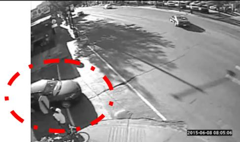
Motorist stops with vehicle completely encroaching into the crosswalk; pedestrian travel path requires significant deviation including possible crossing behind the encroaching motorist, limiting visibility of the crossing pedestrian
