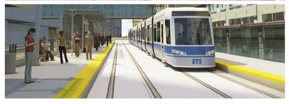
Low-floor LRT vehicles were first introduced in the late 1980s and have since evolved to become the industry standard for new LRT systems in Europe and North America. Most of the mechanical equipment on a low-floor LRT vehicle is located on the roof, which means the train doors open at street level for step-free boarding onto the vehicle.
