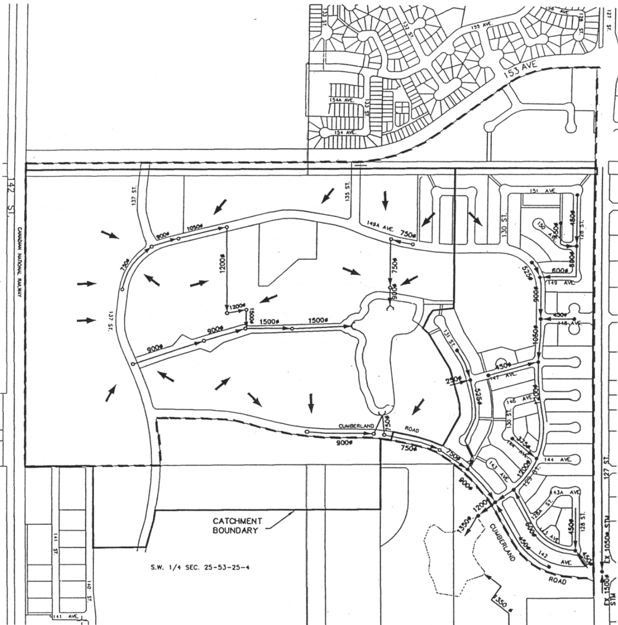
Figure 8: Storm Sewer (Bylaw 11519, June 17, 1997)
