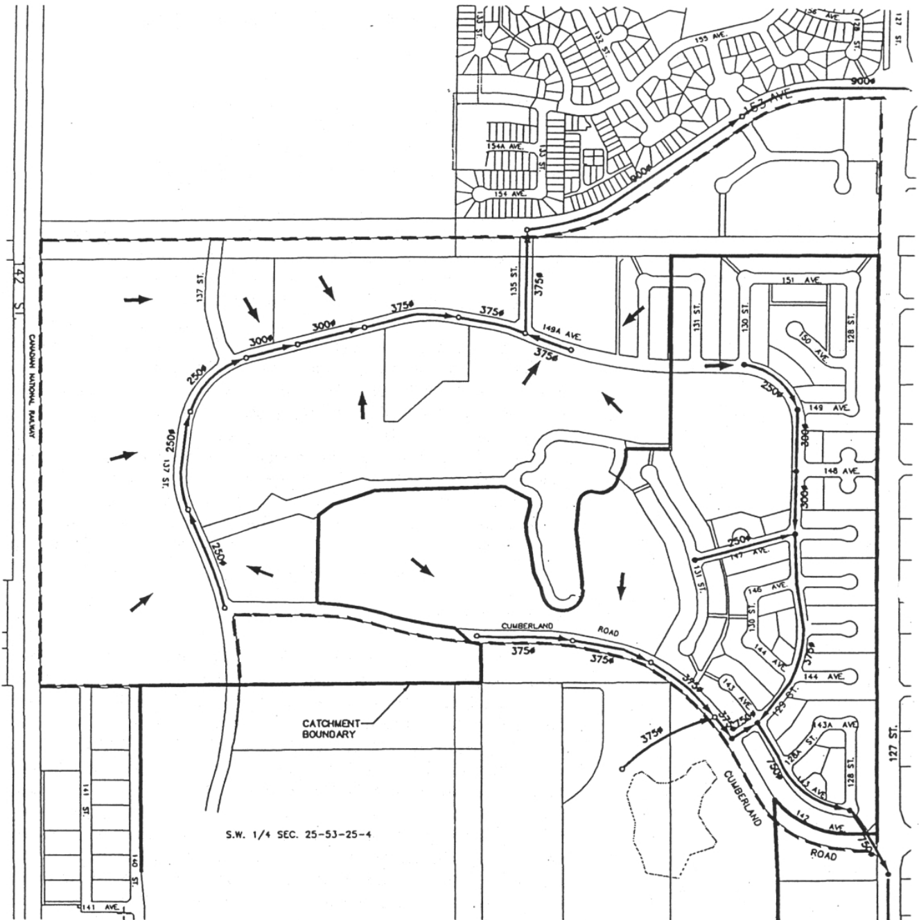
Figure 7: Sanitary Sewer (Bylaw 11519, June 17, 1997)
