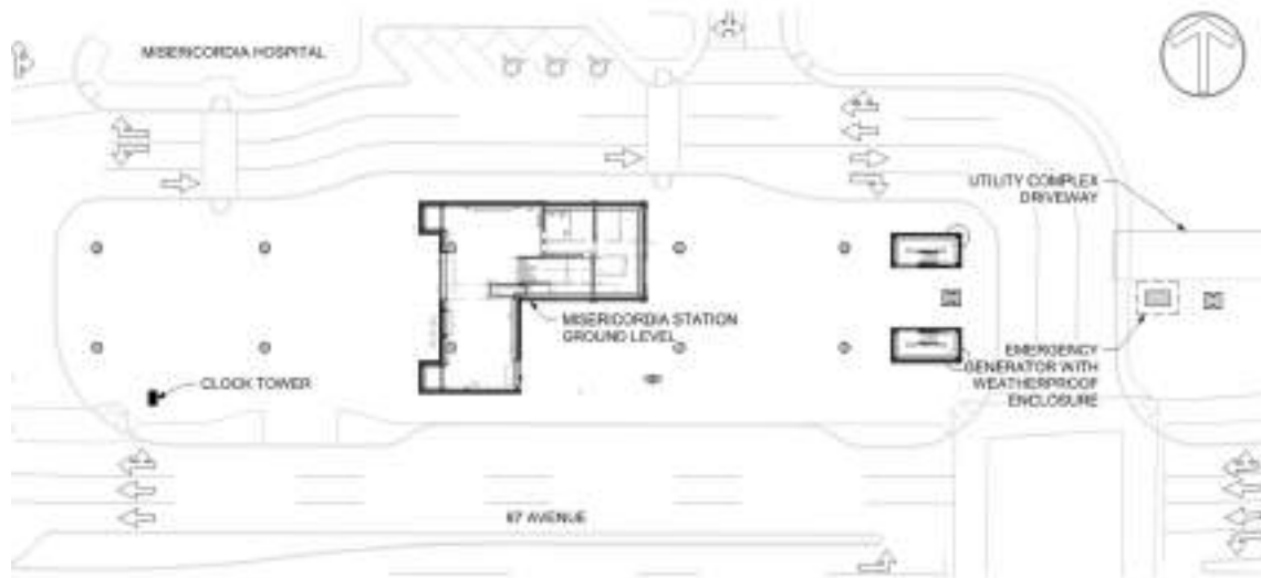
Figure 2-10.3.6F: Misericordia Station Emergency Generator Location
