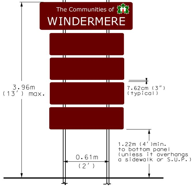
15.24cm x 15.24cm (6" x 6") Pressure Treated Posts -- 2.44m (8') deep. Holes filled with dry sand, compacted in 30.48cm (12") lifts.
